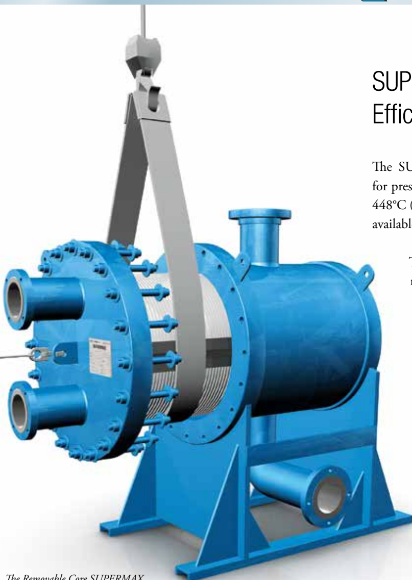
The Removable Core SUPERMAX exchanger is fully accessible on shell side for inspection and/or mechanical cleaning by removing the cover plate assembly.
