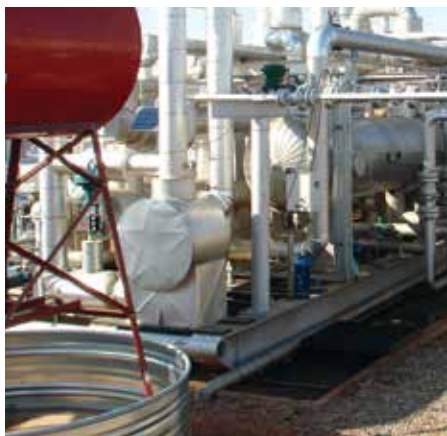
Compact, skid-mounted propane condenser.
