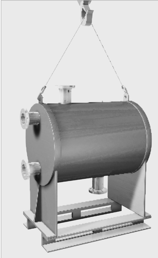
Figure 2.1. Lifting the SUPERMAX exchanger using the lifting lugs. Do not lift the SUPERMAX by the inlet or outlet nozzles.
