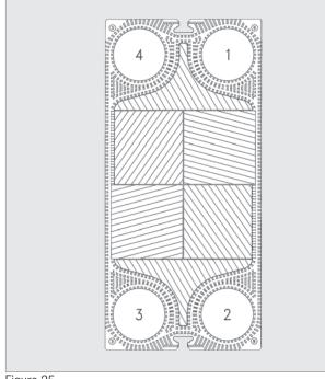
Figure 25 ULTRAFLEX (GX) plate design.
