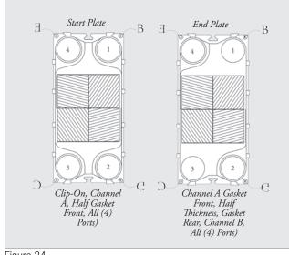
Figure 34 GX Clip-On codes (diagonal flow).
