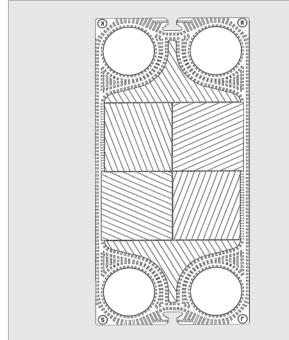
Figure 27 GX type "L" plate.
