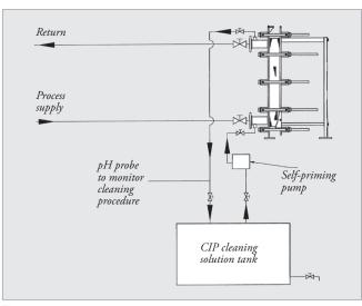
Figure 47 *Cleaning-in-place flow chart.*
