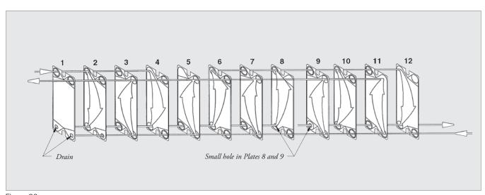
Figure 22 Showing first 12 of the 21 plates in Figure 21 with drains in plates 8 and 9.
