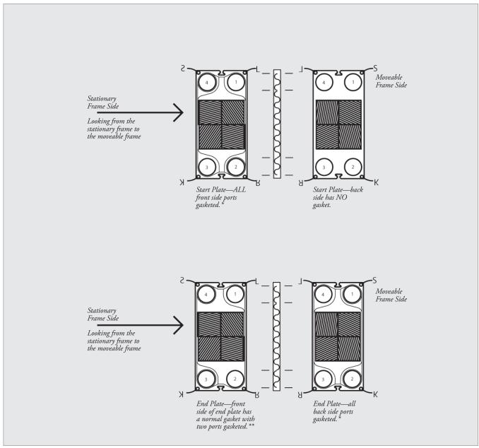
Figure 38 \* These gaskets are half thickness and may be pieced together in various ways depending upon specific model. Flow direction (i.e., Diagonal/Parallel) is not a factor for these gaskets. \*\* This gasket will be the same as all non-Start/End plate gaskets. It will have two ports closed by the gasket. Which ports will be determined by the flow direction (Diagonal/Parallel). Diagonal flow is shown in these illustrations.
