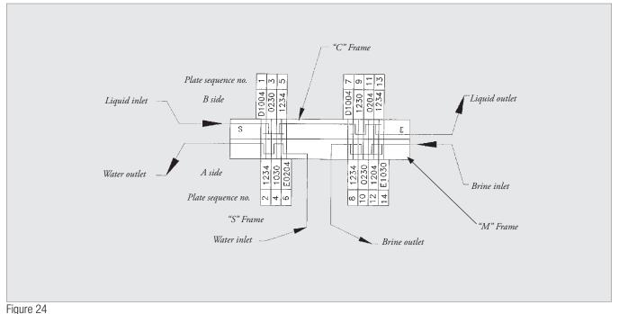
Connecting "C" frame—element composition diagram.
