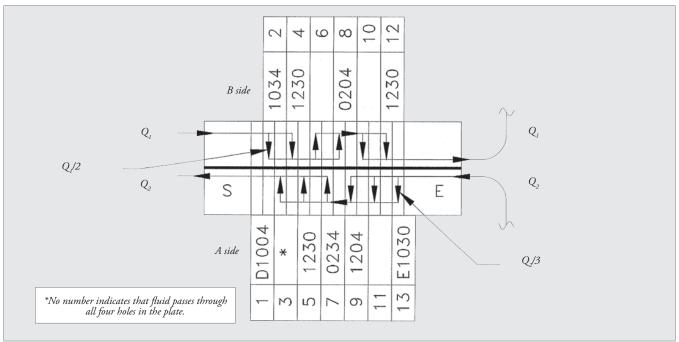
Figure 18 *Flow arrangement.*
