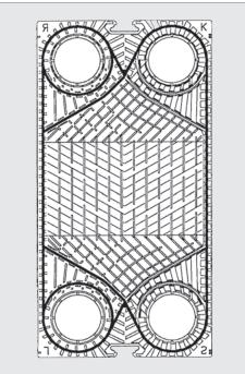
Figure 28 GF-type plate.
