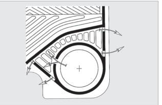
Figure 31 Flow to exterior from damaged boundary gasket.
