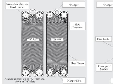
Figure 4 Typical UX, SX, GC or GT Series (herringbone) plate with gasket and hanger. Note that the chevron angle for the herringbone plate can differ on various models.
