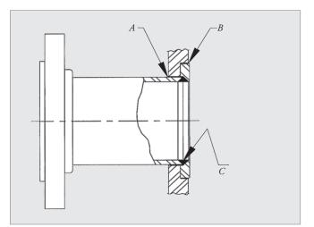
Figure 50 Troubleshooting nozzle/end frame leaks.
