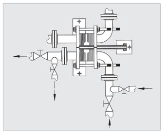
Figure 48 Piping using brine (top view).
