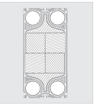
Figure 26 GX type "H" plate.
