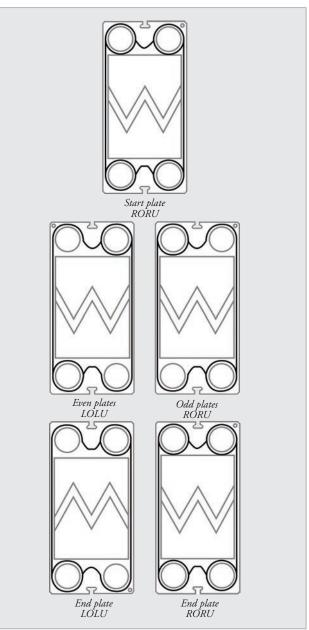
Figure 46 Gasket attaching orientation.
