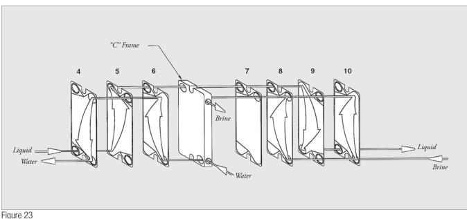
Connecting "C" frame—flow diagram.
