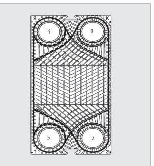
Figure 7 Typical GF (wide gap) plate with gasket.
