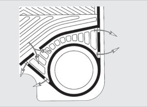
Figure 33 Flow to exterior from damaged boundary gasket.
