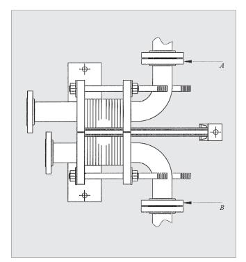
Figure 39 Correct piping installation—disconnecting A and B connections will permit movement of the end frame (top view).
