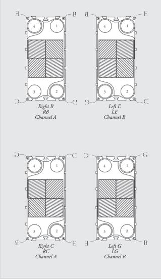
Figure 35 GX Start and End plate explanations.
