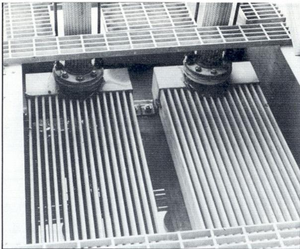
*Fernstrum Gridcooler heat exchangers serve as the cooling system of the engine and gear.*
