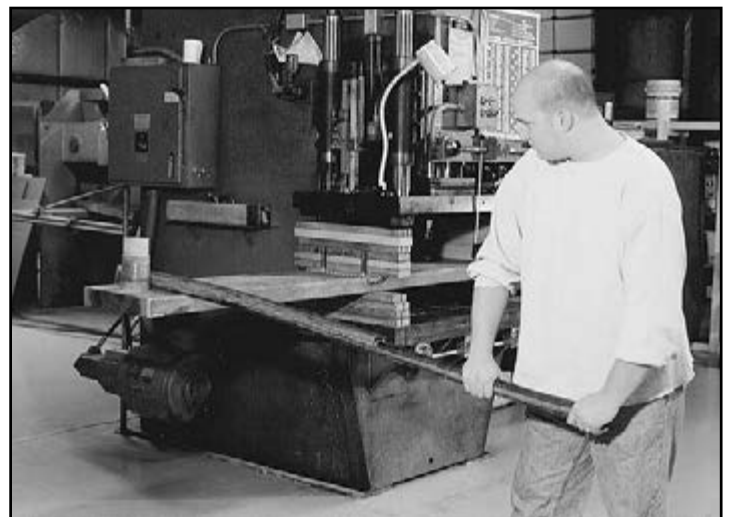
FIG. 26 Carefully apply downward force to impart a twist in the cooler
