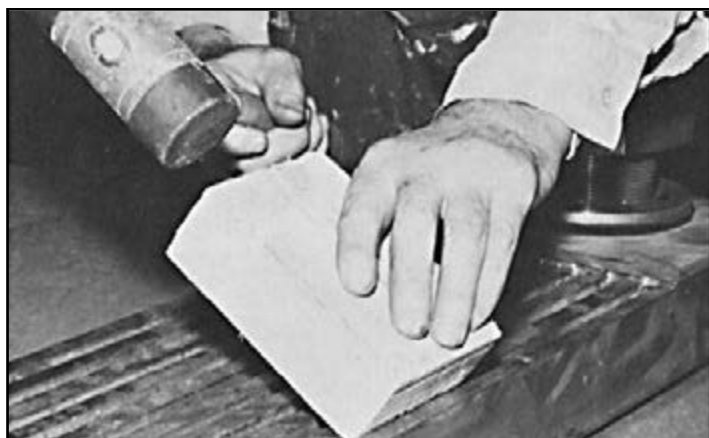
FIG. 27 Straightening tubes with a wooden block & mallet
