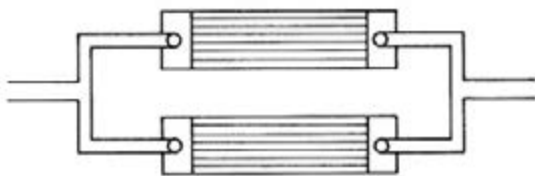
FIG. 13 Coolers connected in parallel
